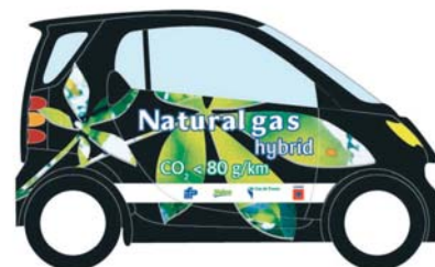
Hybrid natural gas vehicle in which IFP developed the whole ICE-hybrid control system. Partners in the project: ADEME, GDF SUEZ, Inrets, Valeo
